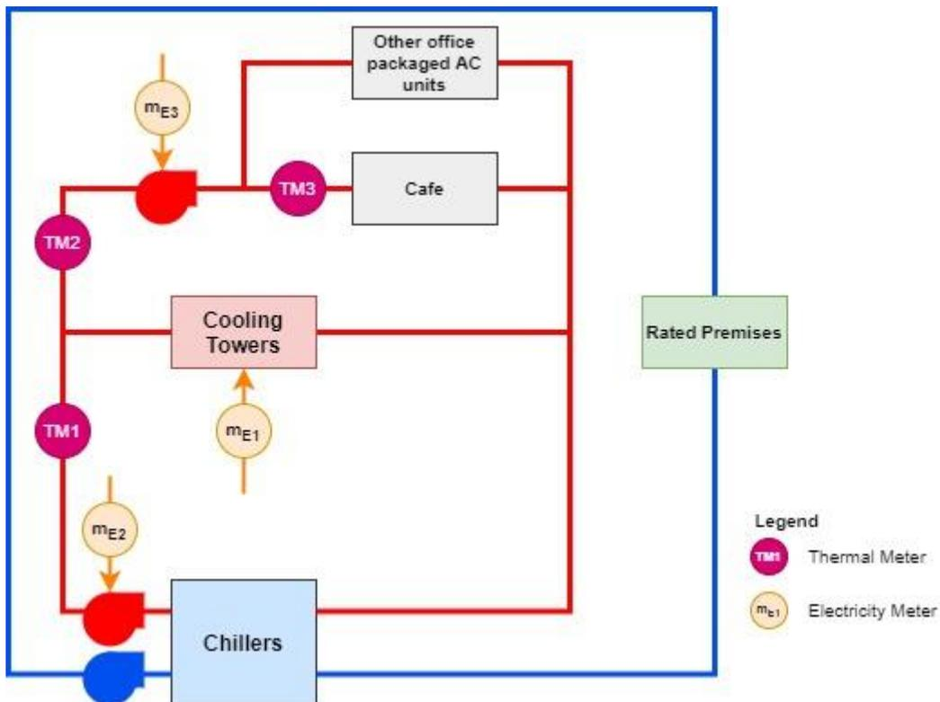
Figure B.7: Example 2 – Condenser water schematic
